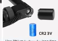
Use lithium battery for long time work, LED low voltage indicator.
